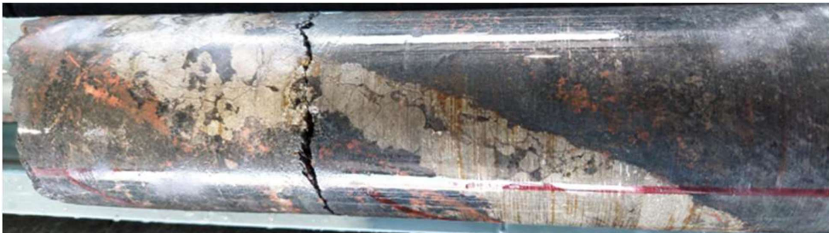
Figure 3: Drill core from 24CNDD05 ~186.5m, quartz vein with pyrite and chalcopyrite
