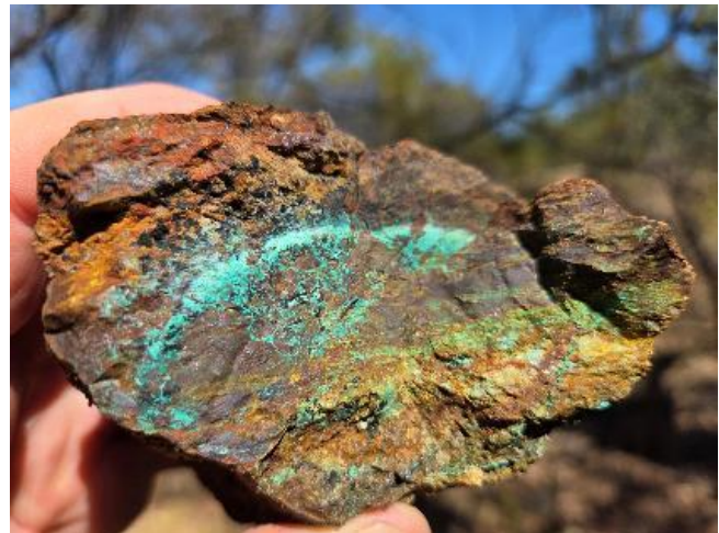
Figure 4: Sample CZR0015 11.7% Cu, 0.09% Pb, 0.28% Zn, 71.7ppm Ag, 0.29ppm Au, 164ppm Bi, 1870ppm Sn
