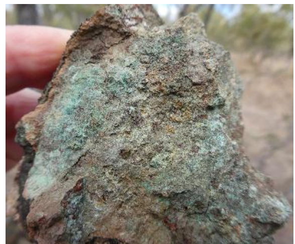
Figure 5: Sample SZR008 10.15% Cu, 0.21ppm Au
