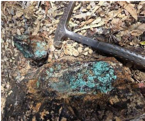
Figure 3: Sample CZR0009 17.9% Cu, 0.61% Pb, 594ppm Ag, 0.36ppm Au, 2170ppm Bi, 1825ppm Sn
